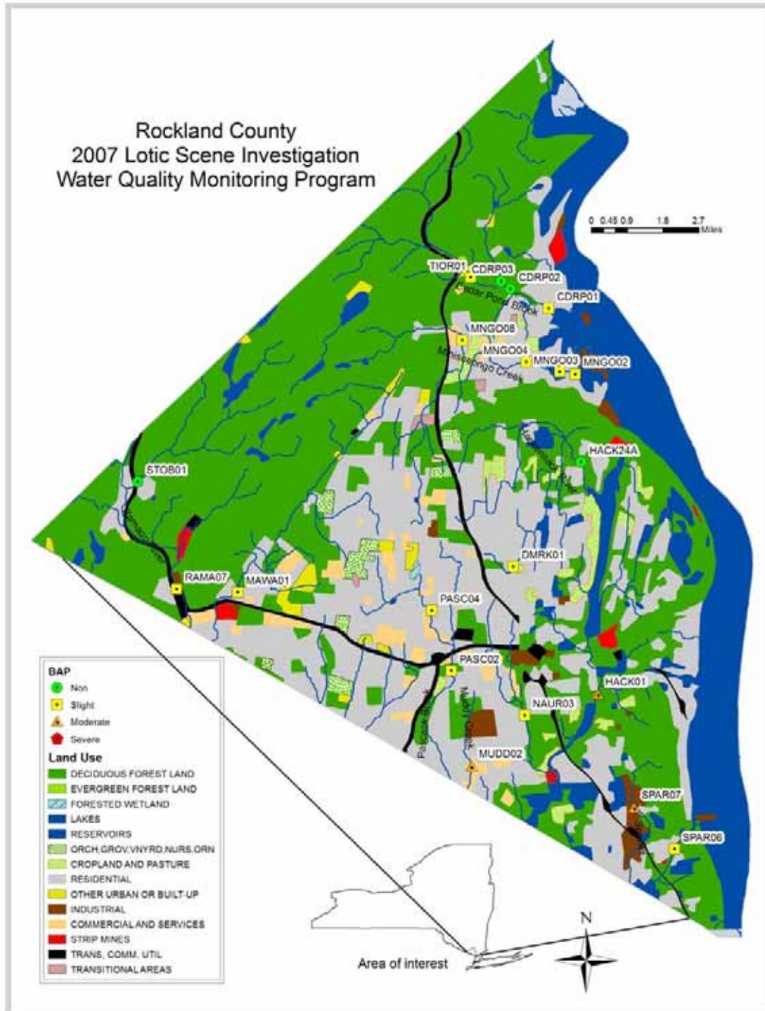
Figure 1. Biotic assessment score (BAP) water quality classifications for the 20 stream stations sampled in Rockland County, NY in relation to land use.
